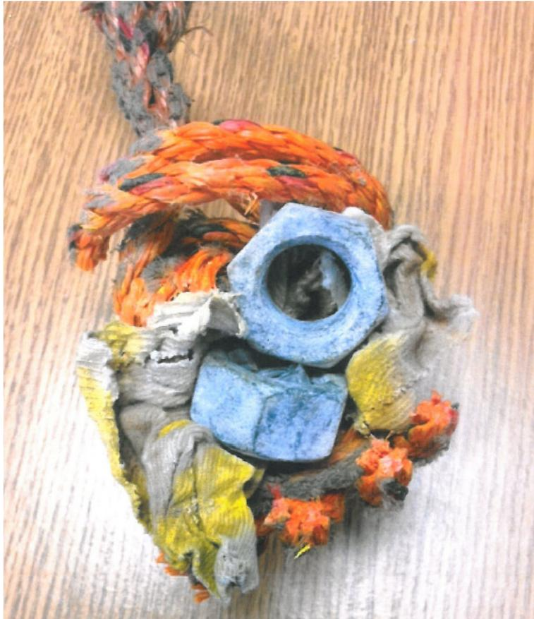
6. Shore mooring teams and Tug Masters have instructions to cut off weighted “monkeys fists” or any added or replacement weights from heaving lines, if used. The weighted “fist” or added weight will be retained as evidence in the event of proceedings being taken against the vessel and the user.
